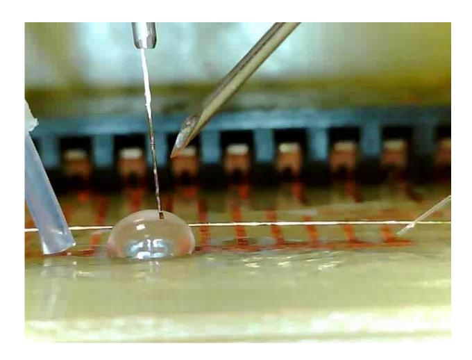
Unique technology for creating microdroplets suitable for portable automatic analytical devices
