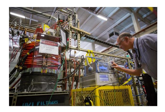
In a diligent, two-month-long process, SLAC engineers tested the first of the XL4 klystrons built for PAL. Credit: SLAC National Accelerator Laboratory
