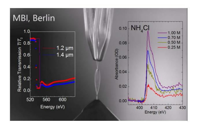
Liquid flatjet system, showing the two nozzles from which two impinging single jets form a 1 mm wide and 5 mm long liquid water sheet with a thickness of 1 - 2  $\mu$ m as determined by measuring the transmission at the oxygen K absorption edge (left), with which XAS measurements in transmission can be made on aqueous solutions, as exemplified with the nitrogen K absorption edge spectrum of ammoniumchloride (right). Credit: MBI
