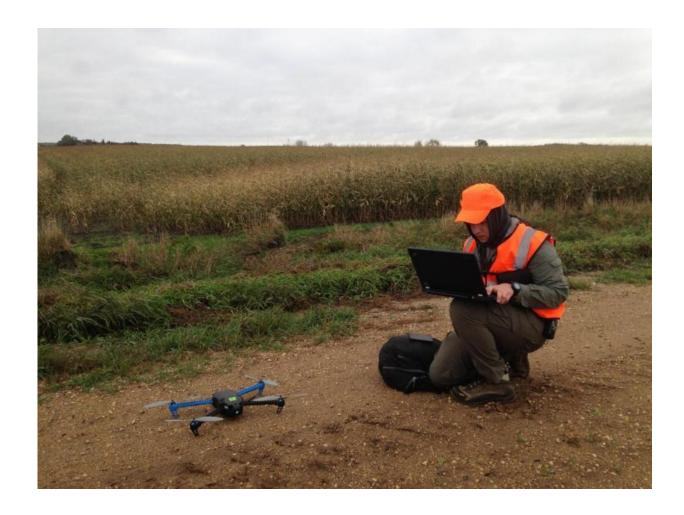
Mark Ditmer downloads the current GPS coordinates of a collared bear to input into a UAV mission. The bear's location is emailed every 2 minutes via Iridium satellite-capable GPS collars, and the researchers programmed the UAV to fly to the most recent location of the bear. Credit: Jessie Tanner (@jessiectanner)
