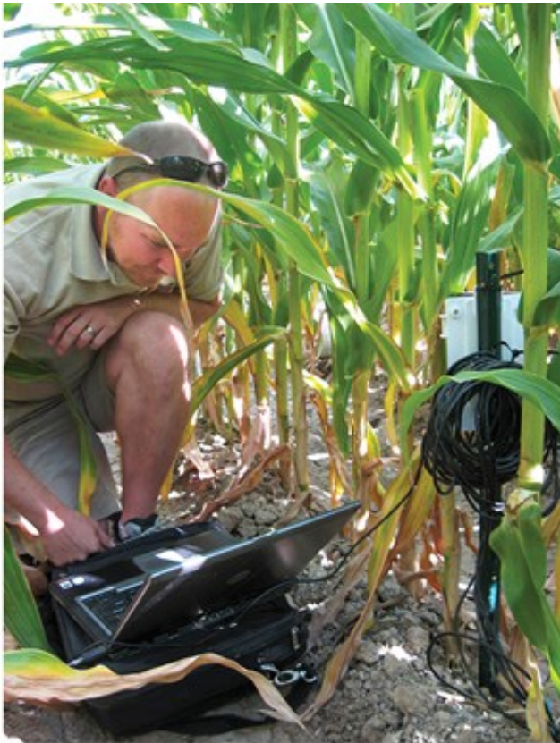
Agricultural engineer Kendall DeJonge, with the ARS Water Management Research Unit, downloads canopy temperature data at a research plot near Greely, Colorado. Grace Lloyd Miner (D3457-1)
