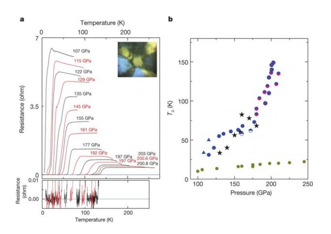
Temperature dependence of the resistance of sulfur hydride measured at different pressures, and the pressure dependence of Tc. Credit: *Nature* (2015) doi:10.1038/nature14964
