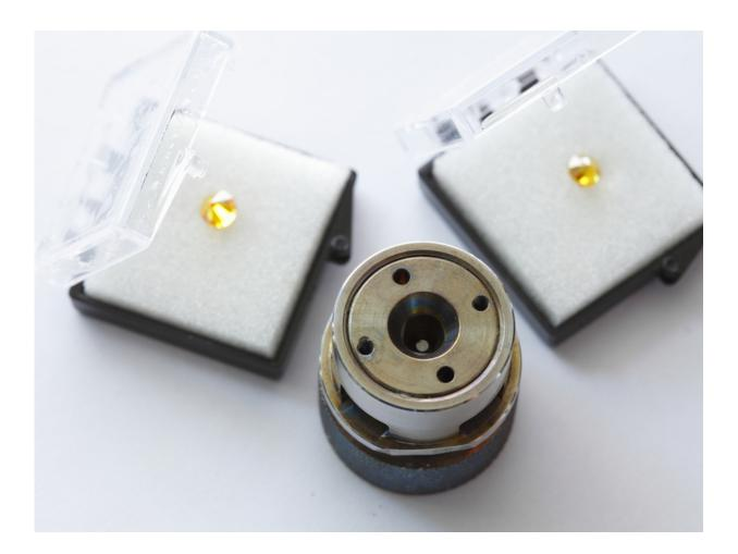
The apparatus the team led by Mikhail Eremets at the Max Planck Institute for Chemistry in Mainz uses to generate extremely high pressures, is amazingly handy. The researchers press the metal cell with Allen screws together. The high pressure thus created in the center of the cell, only diamonds resist. The gems
