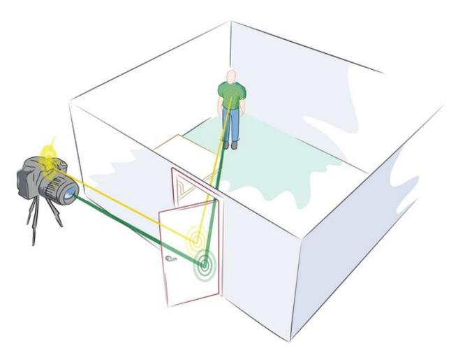
In this example, the imaging system being developed for NASA sends a pulse of laser light off of a surface and into a nonvisible space to "see around a corner." With an ultra-fast flash and high-speed camera, the system can reconstruct images of objects the camera never looked at. Credit: Andreas Velten
