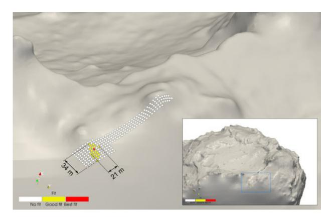
Based on the most recent calculations using CONSERT data and detailed comet shape models, Philae's location has been revised to an area covering 69 x 112 feet (21 x 34 m). The best fit area is marked in red, a good fit is marked in yellow, with areas on the white strip corresponding to previous estimates now discounted. Credit: ESA/Rosetta/Philae/CONSERT
