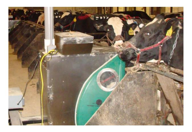
These are Holstein cows being tested for methane production. Credit: Penn State
