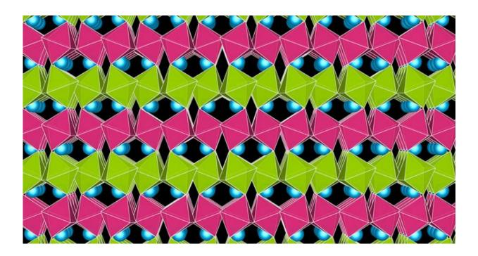
Superlattice structure of lithium osmate and lithium niobate
