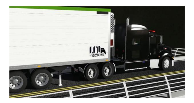
Betting on clean energy sources is the strategy of the Mexican group ISA Tracto C, which produced a series of energetically self-sustained boxes for the transport of perishable goods, with a cooling system that replaced the use of diesel with sunlight and kinetic energy.
