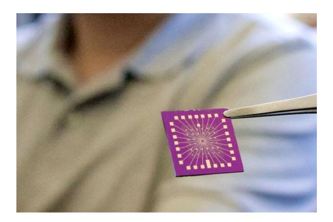
CNSI scientists developed this nanoelectronic chip for use in a new technique called electrical transport spectroscopy. Credit: Tunde Akinloye for CNSI
