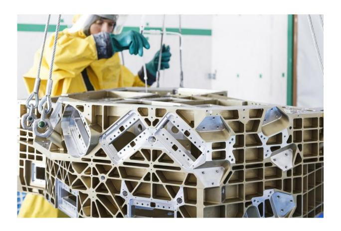
Scientists are regularly preparing instruments for space missions at their cleanroom laboratories. Here, "star attraction" on center stage is the preliminary cleaning of a satellite component. Credit: Fraunhofer IPA
