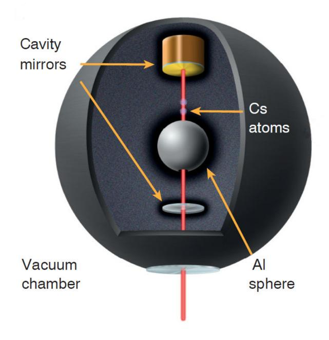
UC Berkeley physicists used an atom interferometer to try to detect anomalous forces from a chameleon field, a hypothetical dark energy particle. If chameleons exist, they would have a very small effect on the interaction between cesium atoms and an aluminum sphere. The group's failure to detect this effect narrows the search for the particle. Credit: Holger Muller/UC Berkeley
