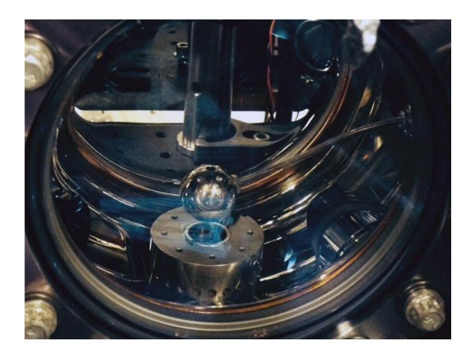
The vacuum chamber of the atom interferometer contains a one-inch diameter aluminum sphere. If chameleons exist, cesium atoms would fall toward the sphere with a slightly greater acceleration than their gravitational attraction would predict. Credit: Holger Muller
