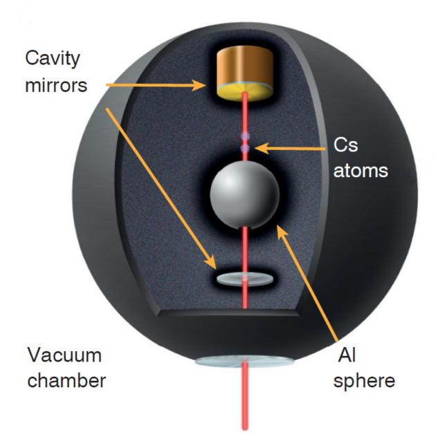
UC Berkeley physicists used an atom interferometer to try to detect anomalous forces from a chameleon field, a hypothetical dark energy particle. If chameleons exist, they would have a very small effect on the interaction between cesium atoms and an aluminum sphere. The group's failure to detect this effect narrows the search for the particle. Credit: Holger Muller/UC Berkeley
