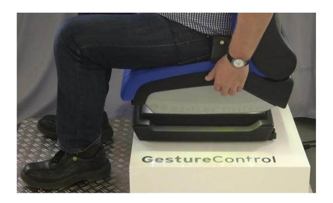
Ease into the correct seat position: with the new seat model, a few hand gestures at the side panel are all you need. Credit: Isringhausen GmbH
