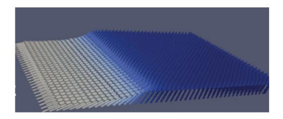
This image taken from a computer simulation shows nanomagnets tilted at various angles, with the white regions indicating greater angles of tilt.
