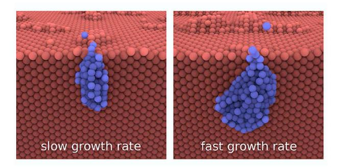
Simulation snapshots of the helium bubble just before bursting. Colors indicate tungsten atoms (red) and helium atoms (blue).
