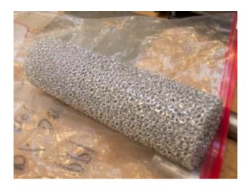
The "steel sponge" in the Lynx separator is made up of a complex network of metal, not unlike a stiff metal scrubber that you might use for cleaning pots and pans. Credit: NTNU
