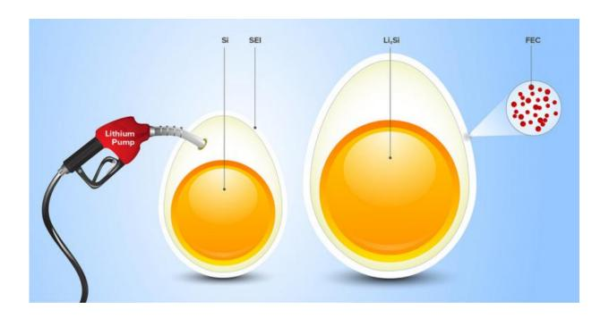
Lithium ions react with silicon to form a new compound, which causes the electrode to expand. Researchers found that flouroethylene carbonate molecules produce a rubber-like protective layer that can accommodate the electrode expansion. Credit: Sana Sandler/Sarah Schlieder
