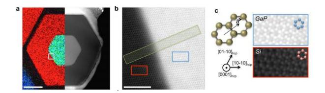
(a) One of the hexagonal nanowires on which the hexagonal silicon was grown.(b) Magnified image of the region marked with a white square in (a). (c)Magnified images of the regions marked with the blue and red boxes in (b), showing the hexagonal structures. Credit: Hauge, et al. ©2015 American Chemical Society
