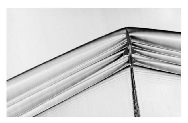
NASA is using a 21st century version of schlieren imagery, invented by a German physicist in 1864, to visualize supersonic flow phenomena with full-scale aircraft in flight. Credit: NASA Photo
