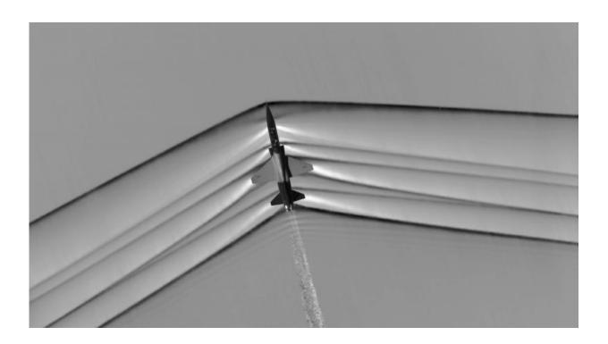
This schlieren image dramatically displays the shock wave of a supersonic jet flying over the Mojave Desert. Researchers used NASA-developed image processing software to remove the desert background, then combined and averaged multiple frames to produce a clear picture of the shock waves. Credit: NASA Photo
