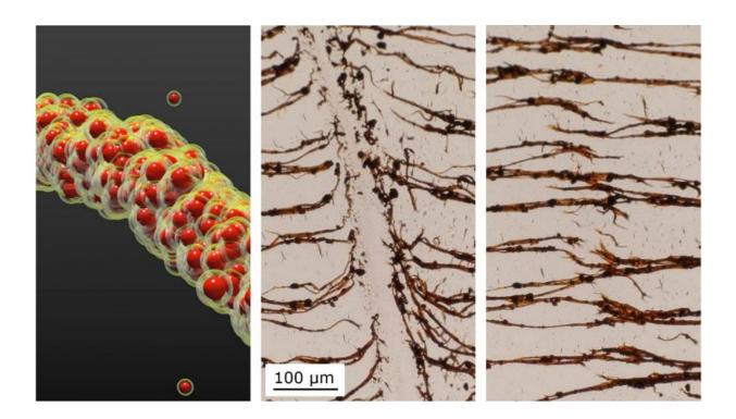
NC State researchers develop a technique to assemble nanoparticles into filaments (left) in liquid. The filaments can be broken (middle) and then re-assembled (right). Credit: Bhuvnesh Bharti.
