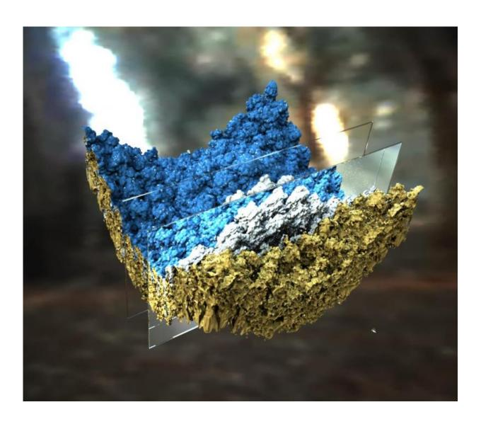
The image shows the turbulent mixing of two fluids in a Richtmyer-Meshkov instability problem, where fluids of different densities are accelerated simultaneously. The photorealistic shading provided by ray tracing makes the
