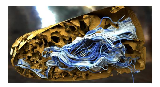
The image shows the path of water through the karst limestone structure of a ground sample taken from south Florida. The photorealistic shading enhances the analysis of the stone porosity and the spatial arrangement of the flow traces. Credit: Data courtesy of Michael Sukop, Sade Garcia, Florida International University and Kevin Cunningham, United States Geological Survey. Visualization: Carson Brownlee, Aaron Knoll and Paul Navratil, Texas Advanced Computing Center
