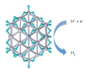
First-principles simulations reveal distribution of absorbed hydrogen atoms (cyan) on a small platinum nanoparticle catalyst during hydrogen evolution reaction. Credit: American Chemical Society
