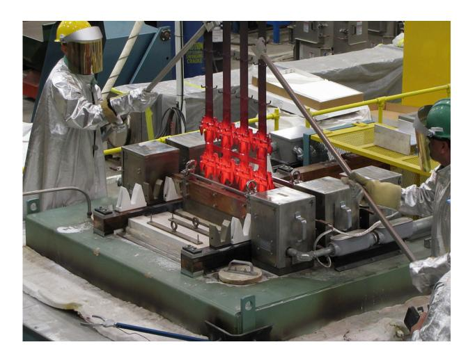
Argonne researchers Osman Eryilmaz (left) and Gerald Jeka (right) recover industrial parts from the large-scale ultra-fast boriding furnace after a successful boriding treatment. This process for extending the lifetime of mechanical parts, which just received its U.S. patent, saves time, money and energy compared to conventional technique, and even alleviates environmental concerns.
