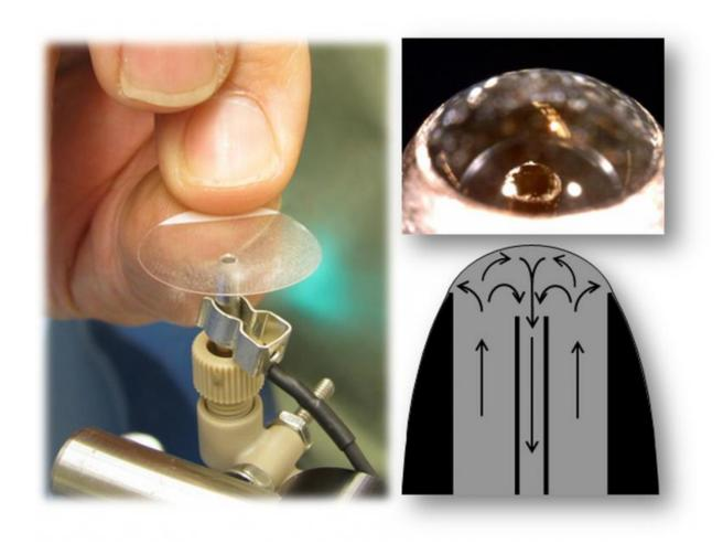
Material dissolved in the liquid at the port tip is immediately transported into the mass spectrometer, ionized, detected and characterized.
