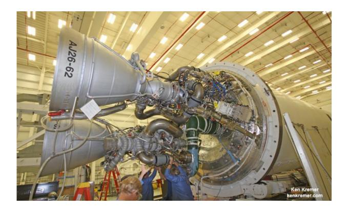
Soviet era NK-33 engines refurbished as the AJ26 exactly like pictured here probably caused Antares' rocket failure on Oct. 28, 2014. Orbital Sciences technicians at work on two AJ26 first stage engines at the base of an Antares rocket during exclusive visit by Ken Kremer/Universe Today at NASA Wallaps. These engines powered the successful Antares liftoff on Jan. 9, 2014 at NASA Wallops, Virginia bound for the ISS. Credit: Ken Kremer – kenkremer.com
