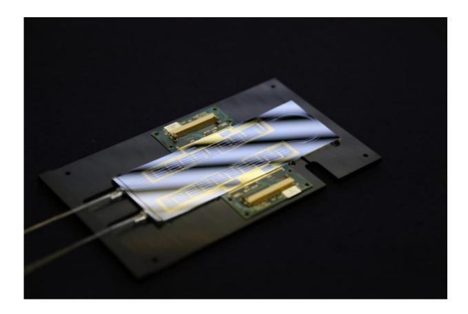
Silicon based quantum optics lab-on-a-chip. Credit: University of Bristol
