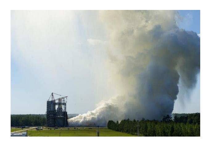
The RS-25 engine fires up for a 535-second test Aug. 27, 2015 at NASA's Stennis Space Center near Bay St. Louis, Mississippi. This is the final in a series of seven tests for the development engine, which will provide NASA engineers critical data on the engine controller unit and inlet pressure conditions. Credit: NASA
