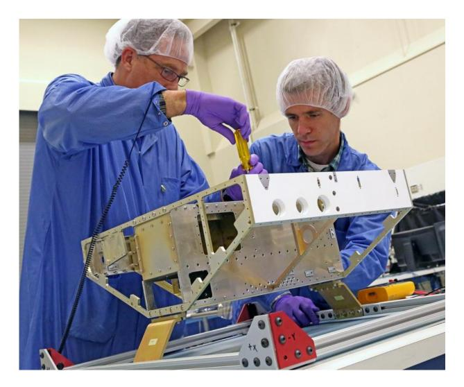
Engineers begin construction of the first of eight microsatellites for NASA's Cyclone Global Navigation Satellite System at the Southwest Research Institute in San Antonio, Texas. Communication antennas, attitude control, GPS receiver, and other instrumentation will be installed on the satellite frame in the coming weeks. Credit: SwRI
