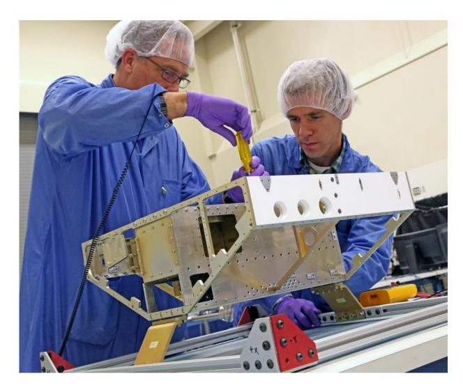
Engineers begin construction of the first of eight microsatellites for NASA's Cyclone Global Navigation Satellite System at the Southwest Research Institute in San Antonio, Texas. Communication antennas, attitude control, GPS receiver, and other instrumentation will be installed on the satellite frame in the coming weeks. Credit: SwRI
