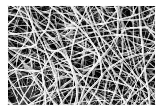
Under a microscope, Nylon-6 fibers comprise nanomembrane sheets.
