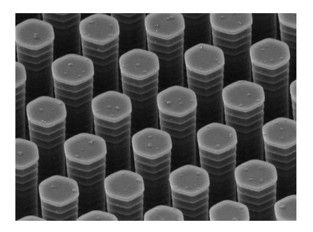
A scanning electron microscope image shows the rigid pillar-like bristles of the FLUENCE rake, which is used to apply light-harvesting polymers to a solar cell. The distance between the pillars is 1 micrometer, about one-hundredth the diameter of a human hair. Credit: Z. Bao et al, Nature Communications
