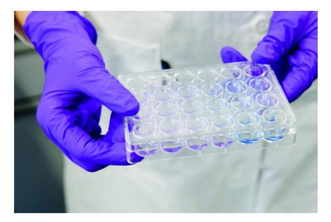
The gill cells are exposed to chemicals in varying concentrations in 24 well plates and their vitality is then analyzed. Credit: © Julian Salinas, ETH-Board
