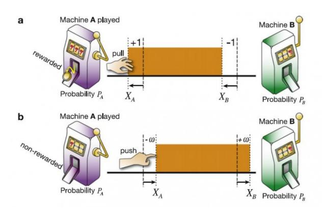
In tug-of-war dynamics, an iron bar can decide which slot machine has the higher winning probability by moving to the left for each rewarded play and to the right for each non-rewarded play of Machine A. The bar's movements are caused by physical fluctuations. Credit: Kim, et al.
