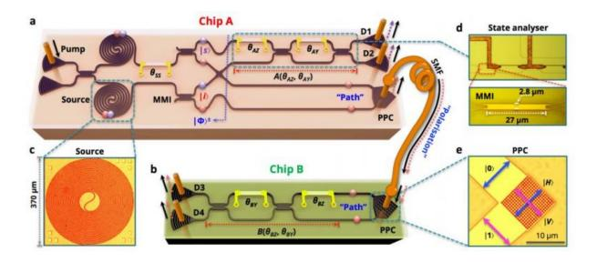
Quantum photonic interconnect and entanglement distribution between two integrated Si photonic chips. Credit: arXiv:1508.03214 [quant-ph]
