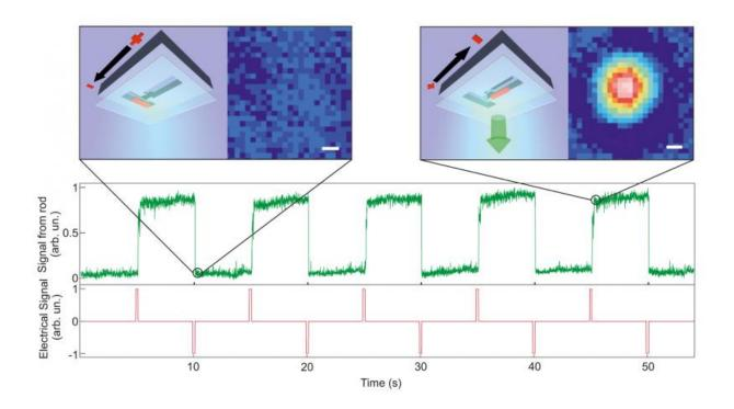
A nanorod is switched between two states – bright (high signal) and dark (low signal) by an external electrical pulse (red trace). The state of the rod can be readout instantaneously at any time using polarized light. The rod stores the most recently written state until the arrival of the next "write pulse."
