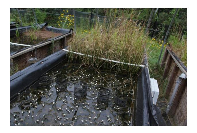
This mesocosm used by the Center for the Environmental Implications of Nanotechnology is basically a small, self-contained ecosystem with embedded sensors that is used to study how nanoparticles interact with all aspects of a natural system. Credit: Duke University
