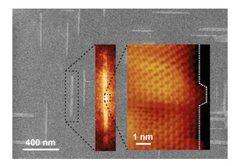
Progressively zoomed-in images of graphene nanoribbons grown on germanium. The ribbons automatically align perpendicularly and naturally grow with their edges oriented along the carbon-carbon bond direction, known as the armchair edge configuration. Credit: Arnold Research Group and Guisinger Research Group
