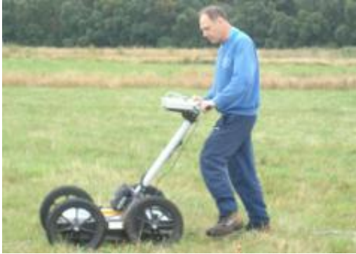
Petr Masters using ground penetrating radar
