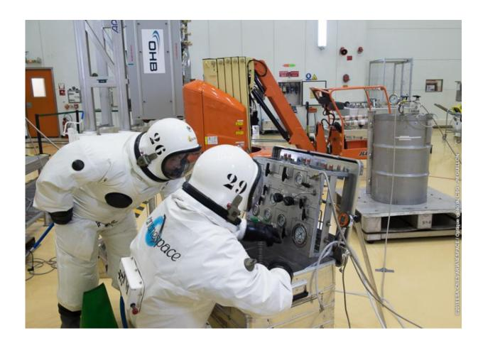
Europe's ninth and tenth Galileo satellites being fuelled by technicians in protective SCAPE suits within the Guiana Space Centre's 3SB preparation building on 24 August. This left them ready to be attached to their launcher
