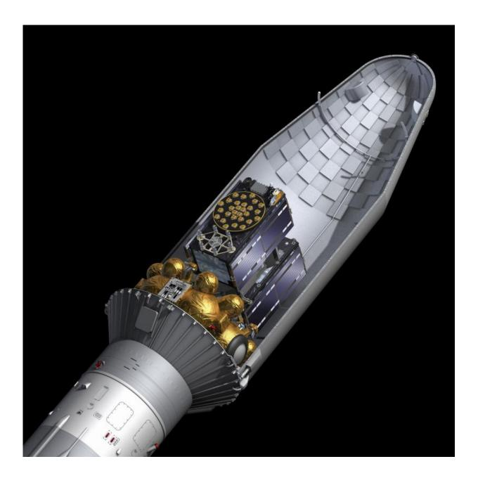
Cutaway view of the Soyuz rocket fairing carrying a pair of Galileo satellites. Credit: ESA–J. Huart, 2014
