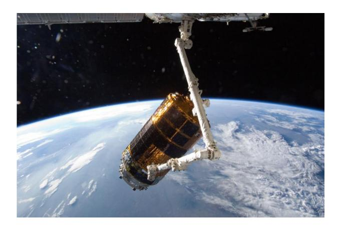
The Japan Aerospace Exploration Agency's (JAXA) H-II Transport Vehicle (HTV)-5 will rendezvous with the International Space Station on Aug. 21. Rendezvous and grapple will occur at 7:55 a.m. EDT, when the cargo craft will be captured by the space station's Canadarm2, as seen in this image when HTV-3 arrived at the space station on July 27, 2012. Credit: NASA
