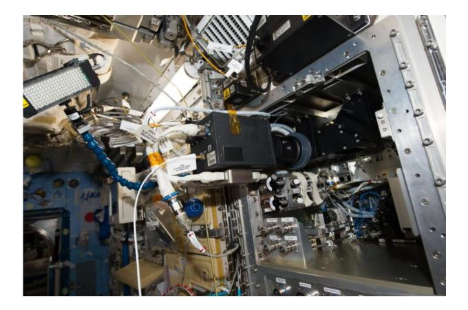
The Japan Aerospace Exploration Agency's (JAXA) Dynamic Surf investigation is looking in to a phenomenon called Marangoni convection -- one of the fundamental principles of liquid motion which is revealed much more clearly in microgravity. Understanding the physics of this convection will improve research in crystals used for semiconductors and optics, and in DNA examination on the space station and on Earth. Credit: NASA
