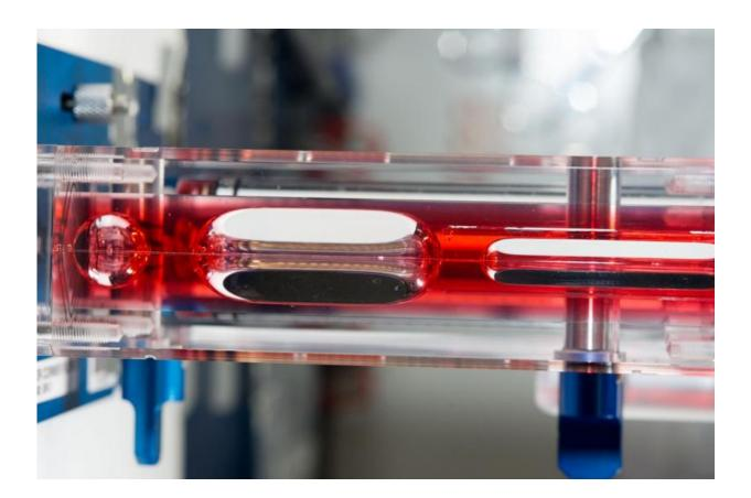
A view of a Capillary Flow Experiment (CFE) vessel was set up during a test run on the International Space Station. This investigation researches a liquid's ability to spread across a surface, and its impact in larger and various container shapes in microgravity environments. This work will improve our ability to quickly and accurately predict how related processes occur, allowing us to design better fuel tanks and water processing systems for life support. Credit: NASA
