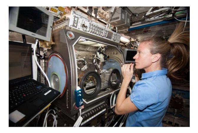
NASA astronaut Karen Nyberg works with the InSPACE-3 experiment in the Microgravity Science Glovebox (MSG) on the International Space Station. InSPACE-3 applies different magnetic fields to vials of colloids, or liquids with microscopic particles, and observes how fluids can behave like a solid. Results may lead to improvements in the strength and design of materials for stronger buildings and bridges. Credit: NASA
