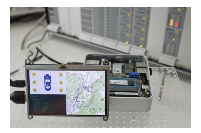
The head unit demonstrator protects manufacturer data as well as vehicle users' private data by preventing unauthorized extraction. Credit: Fraunhofer SIT
