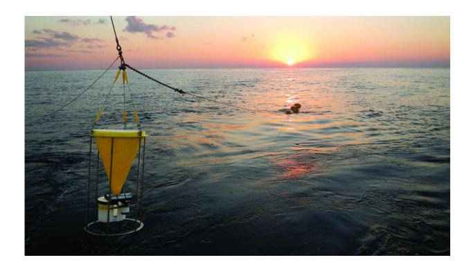
Researchers deployed time-series sediment traps 115 kilometers (approximately 70 miles) southeast of the nuclear power plant at depths of 500 meters (1,640 feet) and 1,000 meters (3,280 feet). The two traps began collecting samples on July 19, 2011 -- 130 days after the March 11th earthquake and tsunami -- and were recovered and reset annually. Credit: Makio Honda, Japan Agency for Marine-Earth Science and Technology
