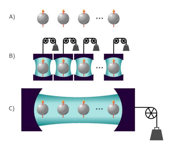
(A) An array of qubits can be charged either (B) in parallel or (C) globally. The results show that, when global entangling operations are allowed on the array during charging, the charging rate increases as the number of qubits increases.
