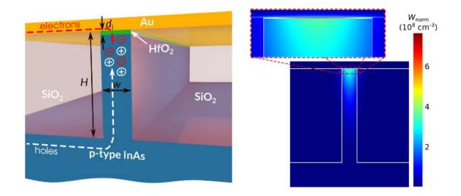
Schematic of the electrically pumped active hybrid plasmonic waveguide and energy density distribution of the surface plasmon field. Credit: Moscow Institute of Physics and Technology
