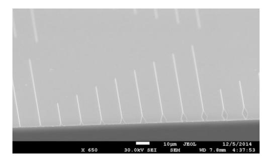
Nanoscale plasmonic waveguides under the scanning electron microscope. Credit: Moscow Institute of Physics and Technology
