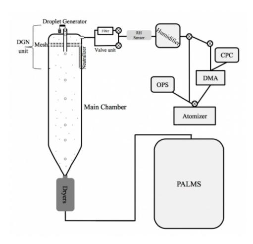
A schematic of the researchers' experimental cloud chamber setup. DGN denotes the droplet generation and neutralizer unit.
