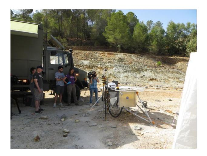
The Life-detection Mars Analog Project (LMAP) rotary-percussive drill, in action during testing. Credit: NASA photo by Brian J. Glass and Carol Stoker
