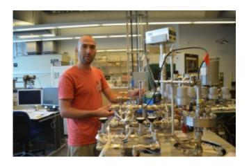
In the lab, with a mass spectometer, used to analyze minute bubbles of gases trapped within diamonds.
